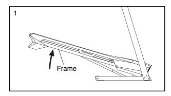
2. Raise the frame until the storage latch locks in the storage position. **CAUTION:** Make sure that the storage latch locks.
