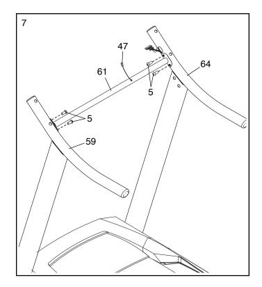
Insert the included tie (C) through the indicated holes in the top and bottom of the Right Handrail (64) as shown. Make sure that the Upright Wire (63) has been secured to the side shown, and then tighten the wire tie.
