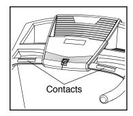
To measure your heart rate, stand on the foot rails and hold the metal contacts on the console. Avoid moving your hands. When your pulse is detected, a heart symbol in the lower right display will flash each time your heart beats, one or two dashes will appear, and then your heart rate will be shown. For the most accurate heart rate reading, continue to hold the contacts for about 15 seconds.
